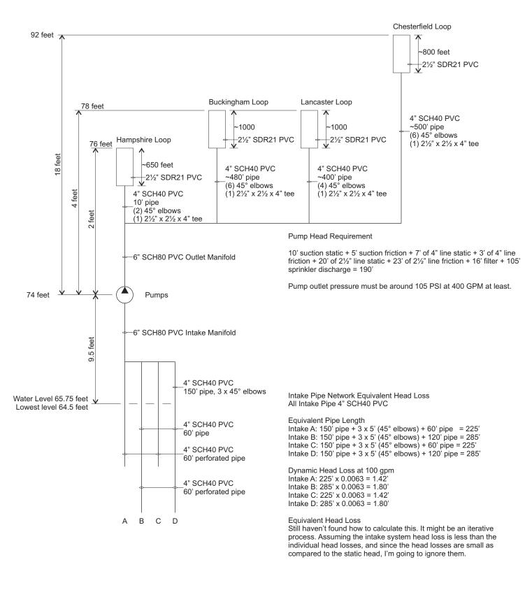
Outlet Pipe Network Equivalent Head Loss
